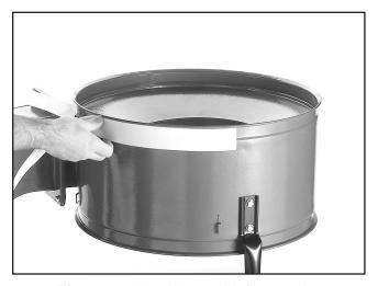
Figure 14. Installing wide foam strip.
